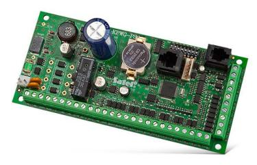
Configuration and some functions of ACCO-KPWG-PS might be different due to the system, which the controller is part of. Within the **ACCO** system the module is programmed by means of an LCD keypad or PC computer with **ACCO-SOFT-LT** software installed. The PC can be connected via RS-232 port or via RS-485 bus using **ACCO-USB** converter. In the **ACCO NET** system, the controller configuration is performed using the **ACCO Soft** software.
