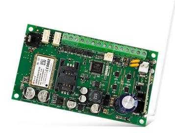
can not only implement SMS notification of events via SMS, but also transmit information to alarm monitoring companies. In addition, **remote operation via SMS** is possible, so you cannot just arm/disarm the system, but you can even control devices connected to the module. The MICRA module, like other SATEL's devices, feature top quality workmanship and well–thought–out technical solutions. This means not only a guarantee of trouble–free operation, but also the appropriate level of security.
