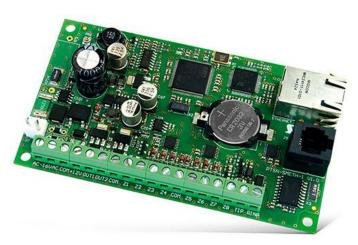
ETHM-2 can be configured remotely via Ethernet or locally via RS-232 port using a computer with the ETHM-2 Soft program. Remote control of the module via a web browser is also possible (only ETHM-2 FLASH v1.02).
