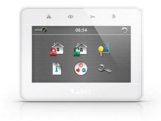
**INT-TSG** also provides an easy access to the information on current system status. Thanks to the status screen customization possibilities, a single glance at the display could be enough to find out if the system is armed, if the outdoor lighting is on or if the garden watering is currently on. The status screen may also be used for the picture gallery.
