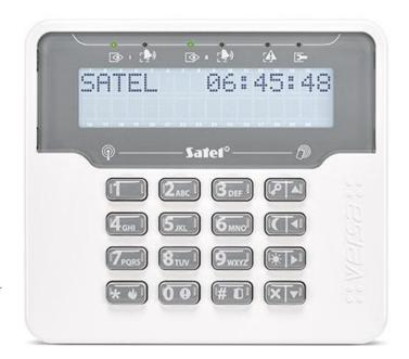
The keypad power source consists of two CR123A 3 V batteries, whose condition is being constantly monitored. The device works in the wake-up or sleep mode (saving energy after 20 seconds of inactivity). For additional reduction of energy consumption, you can disable the proximity card reader (e.g. when it will not be used for operating the alarm system).
